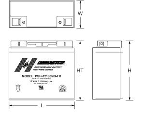
**L**: 7.14 (181) **W**: 3.03 (77) **H**: 6.59 (167) **HT**: 6.59 (167) Tolerances are +/- 0.04 in. (+/- 1mm) and +/- 0.08 in. (+/- 2mm) for
